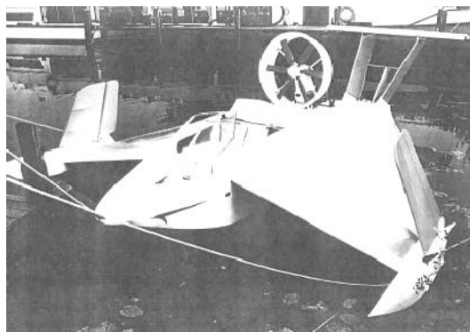
Figure 7 : Notice the foldable "winglets" used for turns, for a better navigation in harbours
