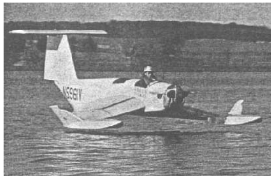
Figure 1 : Note the characteristic negative dihedral along the leading edge
