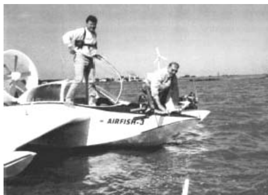
Figure 8 : The AF-3 was later equipped with Power Augmentation for experiments. Her two front propellers can be seen on this picture
