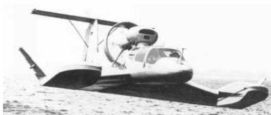
Figure 5 : The catamaran nature of the X-114 is clearly visible on this picture
