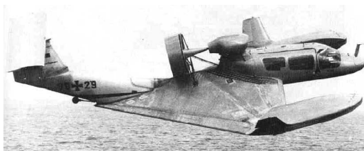
Figure 6 : The X-114 was capable of free flight, as required by the German military authorities
